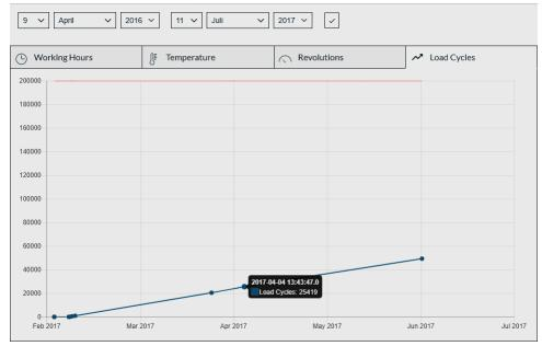
Trend for load cycles (e.g. number of drilled holes): reliable trend with few data sets possible. Detailed data by touch over.
