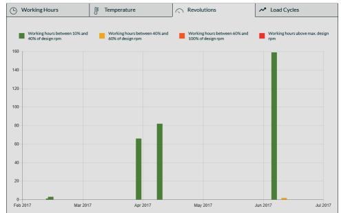
The tool was working mainly between 10 and 40% of the design rpm. Only 2 hours between 40 and 60% of the design rpm. Many more tool related data are to be found in the eltimon cloud.
